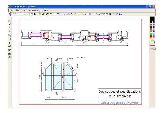
You may predefine drawing models in which the elevation and sections are always inserted in the same locations and include, for example, a footer with the name of your company.
